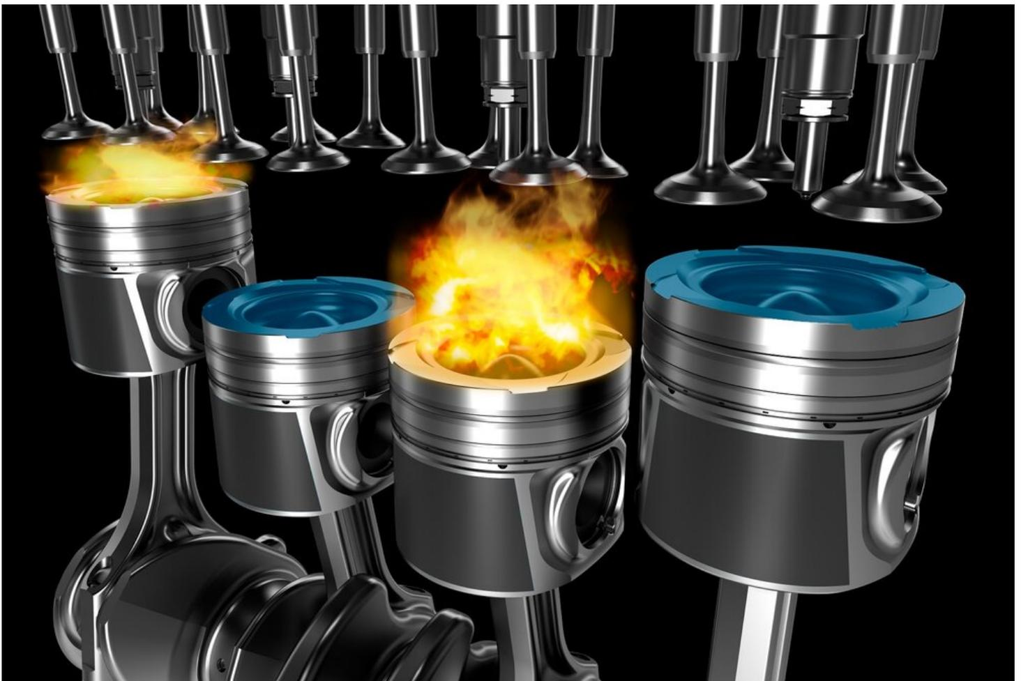
This knock or pinging is the disruption of the delightfully synchronous ballet of sucking, squeezing, banging and blowing - it's upset by virtue of early blowing, which, at high revs and big throttle inputs can destroy your engine. So the designers try to avoid that, sometimes by using a high octane fuel.
