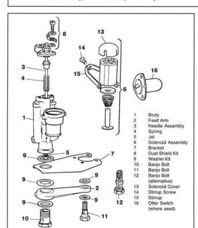
The auxiliary carburetter is used on certain installations to provide automatically differing degrees of mixture enrichment at:
