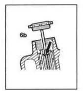
Check the piston damper oil level:
