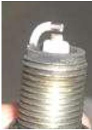
Use a felt marker to mark the ground tip in line with the side of the centre electrode.
