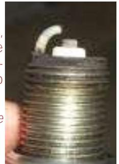
With a small file, carefully smooth edges of the electrode arm to remove any remaining burrs, keeping the edges clean and sharp.
